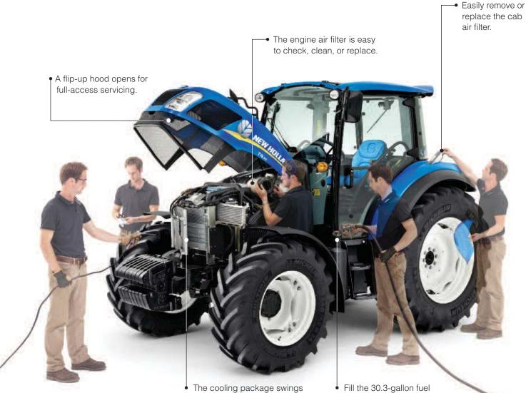
The cooling package swings out to make cleaning faster and easier. • Fill the 30.3-gallon fuel tank from ground level.
