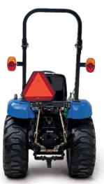
Rear PTO and 3-point hitch allow you to attach countless implements to any job.
