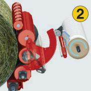
The duckbill pivots into the bale chamber between the fixed roll and pivot roll.
