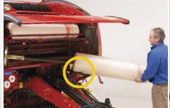
One active roll of net wrap is easily loaded using the net tube.
