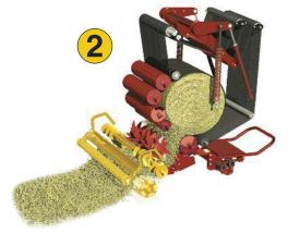
As the bale grows, the top rolls (G & H) pivot forward. The belt tension arm (I) also rotates to allow the bale chamber to expand. The belt tension cylinder (J) and belt tension spring (K) deliver reduced belt tension at the start to ensure positive core formation, even when baling short, dry crop.
