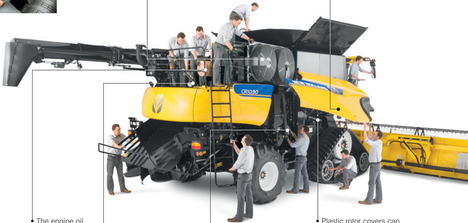
The engine oil and air filter is easy to access from the engine platform.
