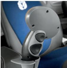
Shift button and ground speed unlock (behind)
