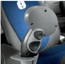
Shift button and ground speed unlock (behind)
