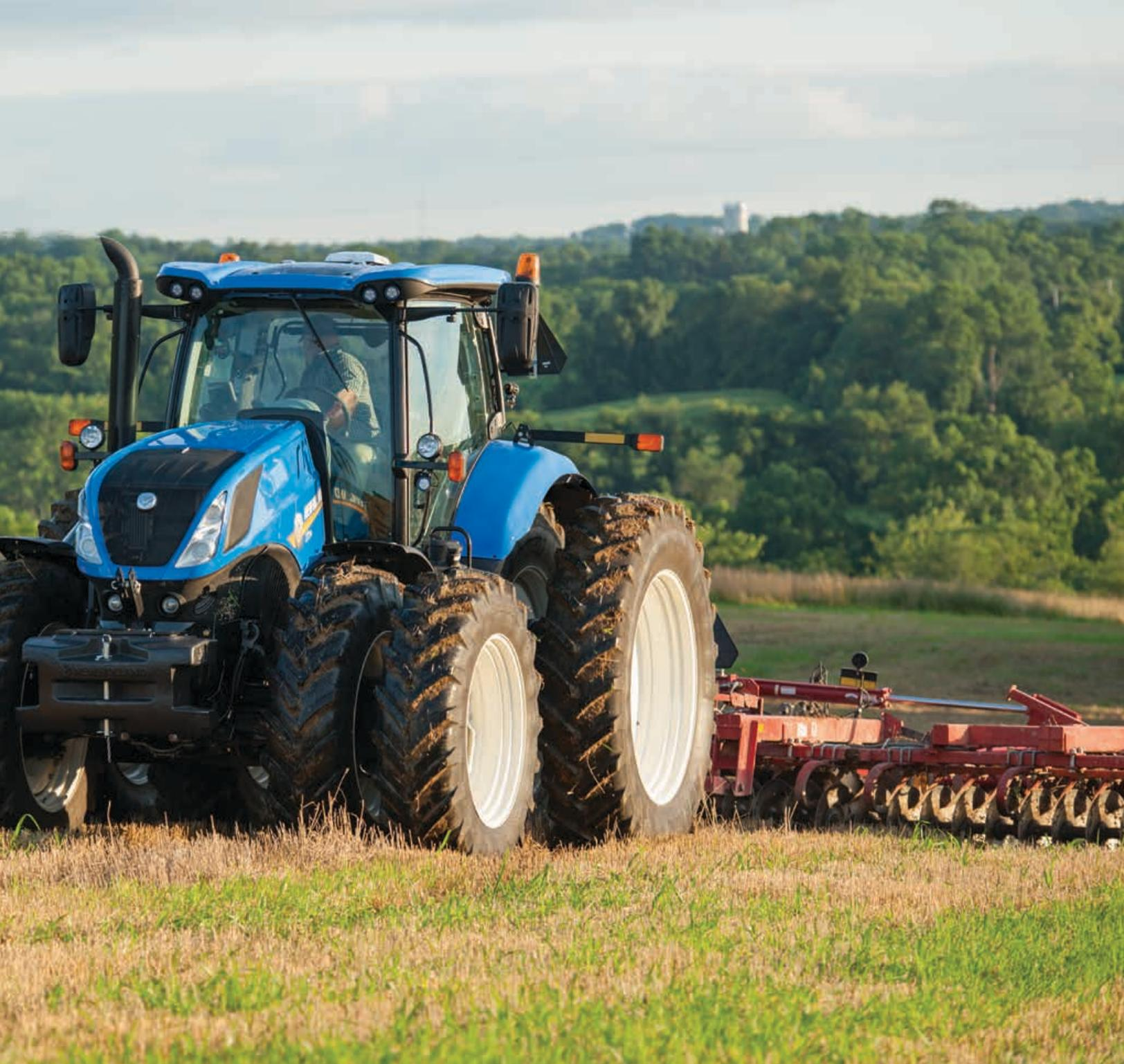
*Rear and front dual wheel options available for field work or large singles for transport.*
